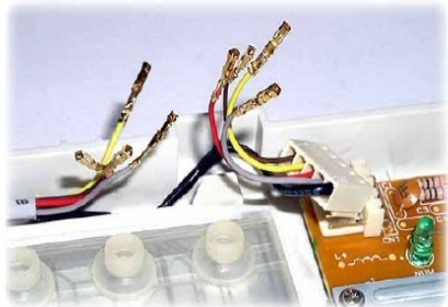
Prepare the wire tips. Crimp the provided connector sockets over the wire tips with the pliers or crimp tool.
